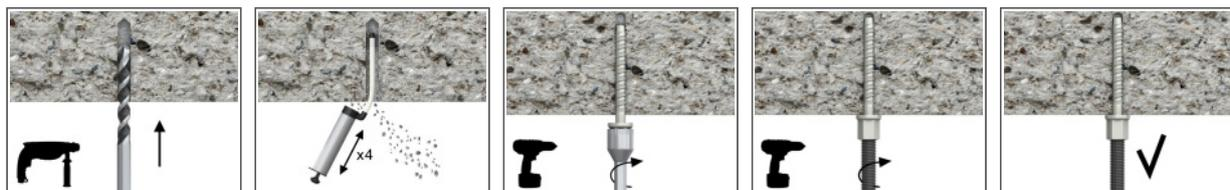
1. Drill the hole with rotary hammer drilling machine. Drill to a required depth.
